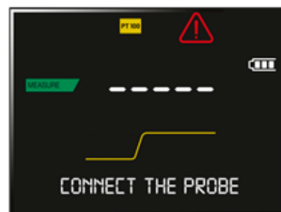
Color backlit LCD display with self-diagnosis messages
