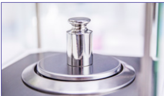
Provided with sample mass (precision class E2) for test and calibration
