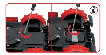
4. Unplug the connector. Replace the old battery with the new one. Then plug the connector.
